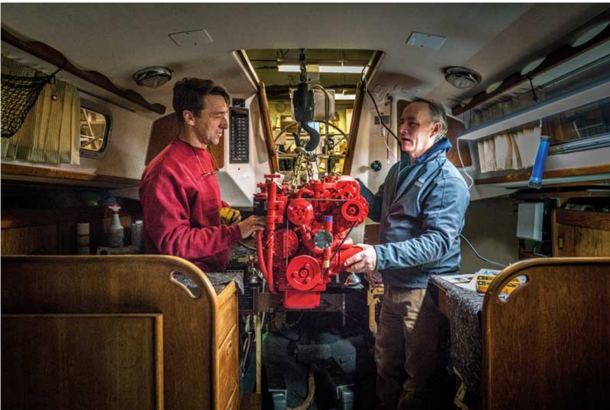
Michael Kunhardt, left, and Neil Collins install a new Beta engine in a Sabre 34. Photo by Heather Perry
